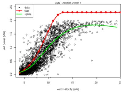
Figure 9 – Power curves for a wind farm: red – manufacturer’s curve; green – approximated spline to the measured wind speed and output unit power (black dots)
